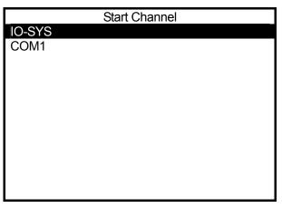
The Drive Control (M), Return to Work Home (R2), and Start (R3) commands are valid only when the start channel is COM1 and the robot is in the run mode.
