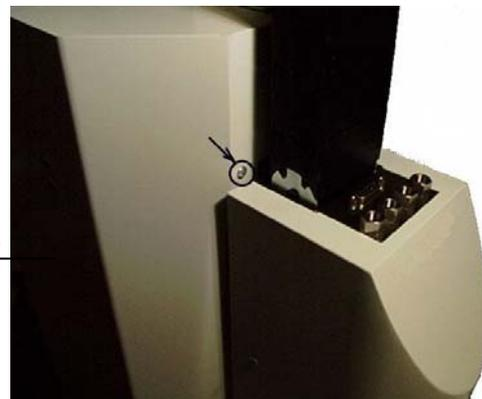
1. Remove the seven screws indicated by arrows to remove the right side cover.
