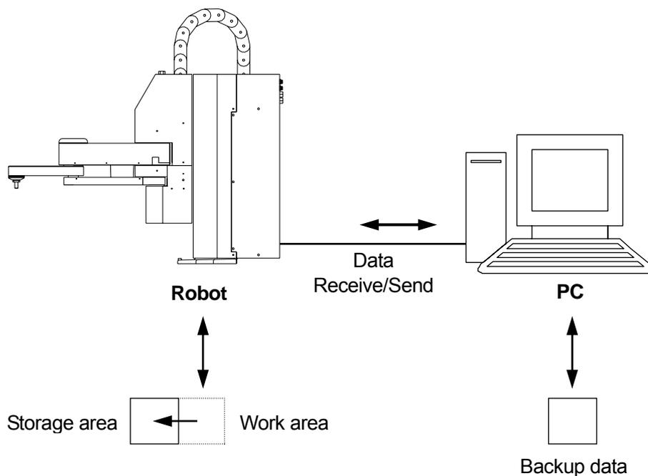
The robot has a data storage area and work area. When you start up the robot, the C & T data in the storage area is copied to the work area. The copied data is used for running and teaching. The data in the work area is deleted if the power to the robot is turned off.
