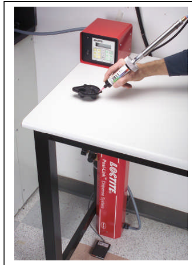
Photo shows a Posi-Link™ Controller (item #98377); Actuator (item # 98378); and Nest Assembly (98645). All items must be purchased separately.
