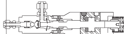
PISTON FULLY RETRACTED, CHECK BALL ON SEAT, METERING CYLINDER IS REFILLED WITH PRODUCT. PUMP READY FOR ANOTHER DISPENSE.
