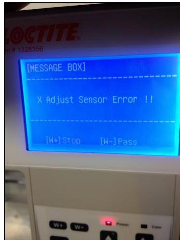
**Figure 6 & 7:** Needle tip is too high in the Z direction, need to lower so it crosses the sensors.
