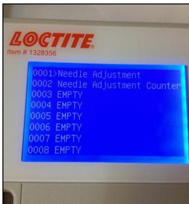
**Figure 7:** This is how the memory address screen will look after programming the Needle Calibration Kit is complete.
