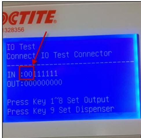
3) Take a dispense needle in your hand. Manually put the needle down in the calibrator and move back and forth in front of the X sensor (right and left). You should see a 1 appear in the first digit when the needle crosses the sensor. See **Figure 8** below. Repeat for the Y & Z sensor (forward and backwards), you should see a 1 in the second digit. See **Figure 9** below.
